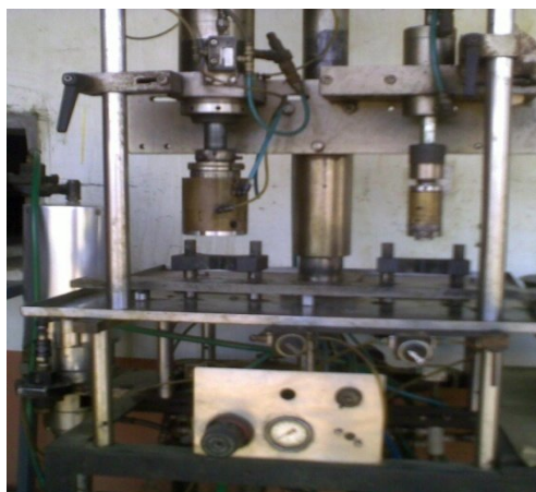
Figure 1: - Aerosol crimping and filling machine.
